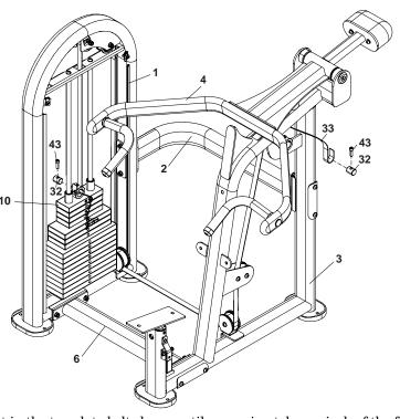
Insert one end of the weight belt (33) through the slot in the top plate belt clamp until approximately one inch of the free end of the belt protrudes from the slot in the opposite side of the clamp.
